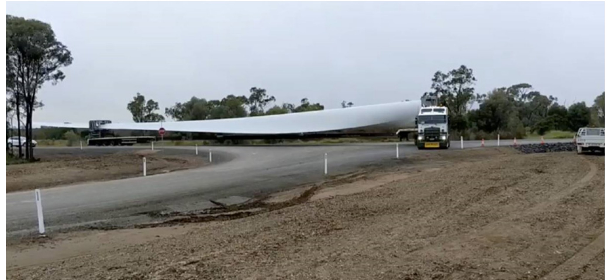
Transportation of 75 m wind turbine blades from Brisbane to Dulacca Wind Farm. Picture source: RES
