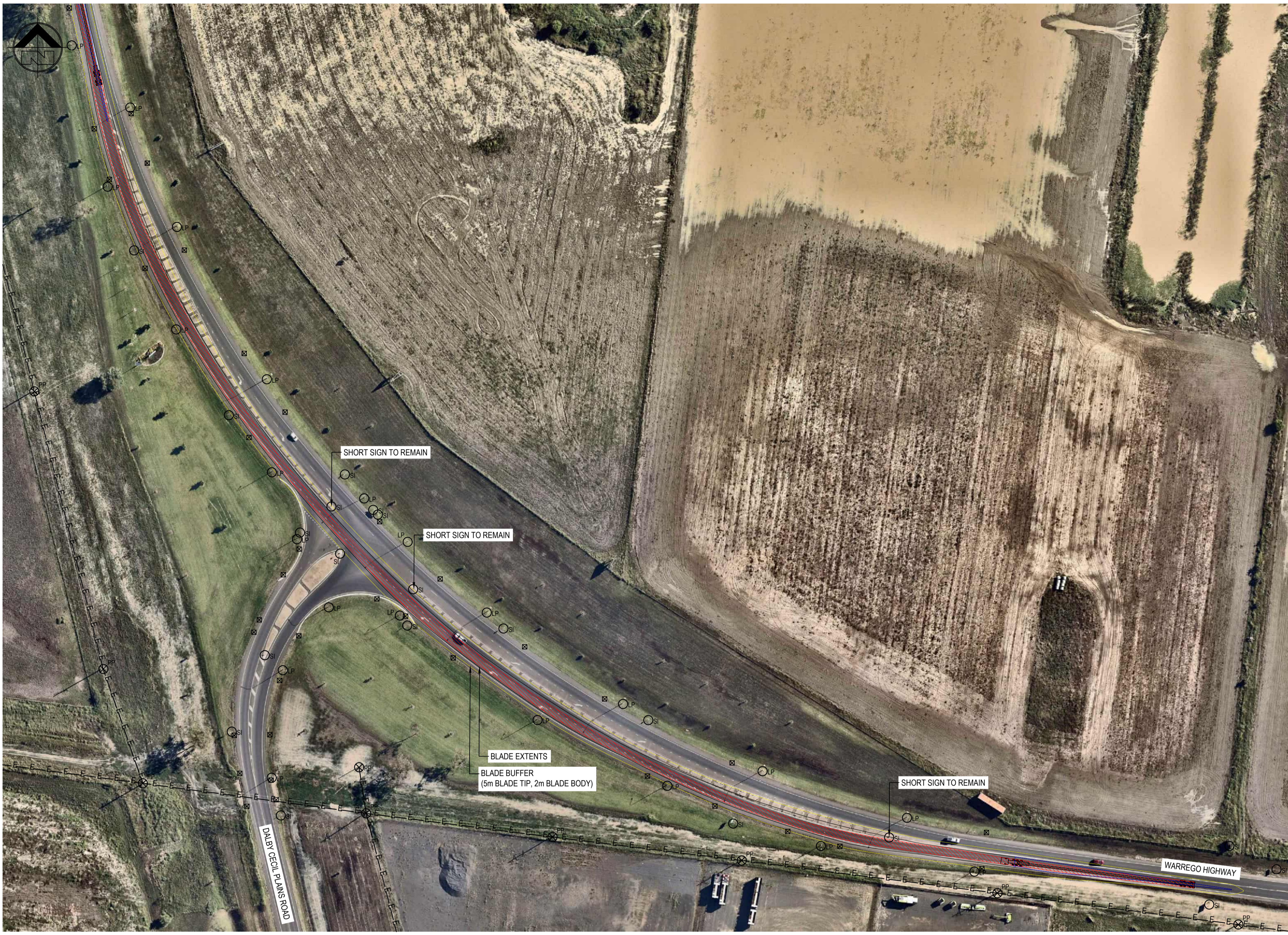
INTERSECTION 8 - WARREGO HIGHWAY / DALBY CECIL PLAINS ROAD INTERSECTION PLAN - 90m BLADE TRUCK AND TRAILER
