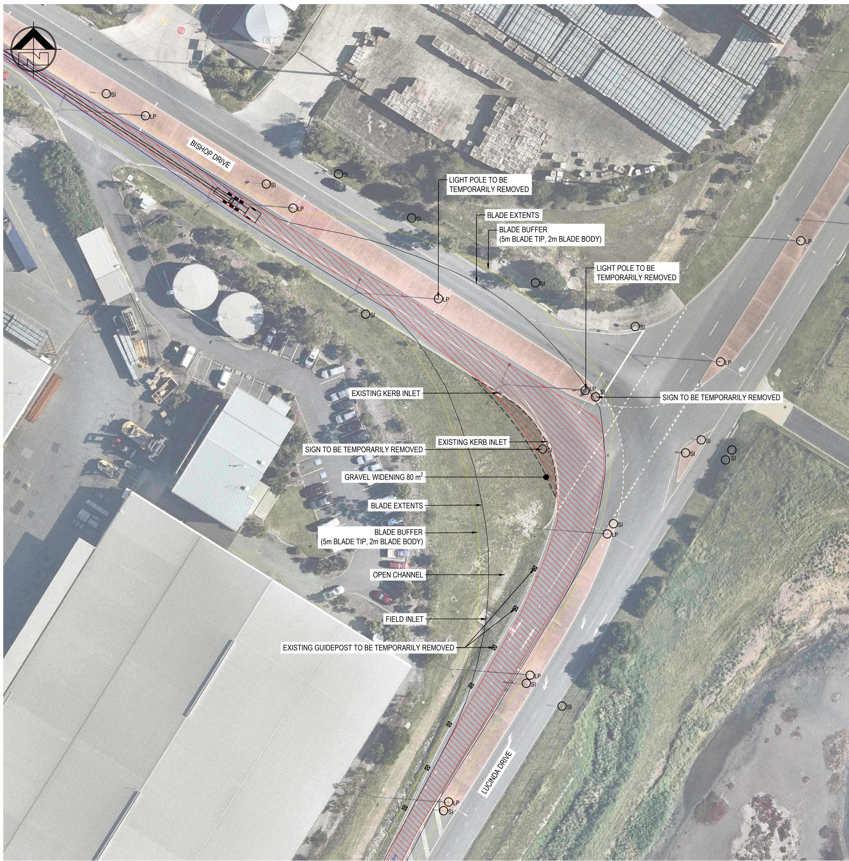
INTERSECTION 1 - BISHOP DRIVE / LUCINDA DRIVE INTERSECTION PLAN - 90m BLADE TRUCK AND TRAILER
