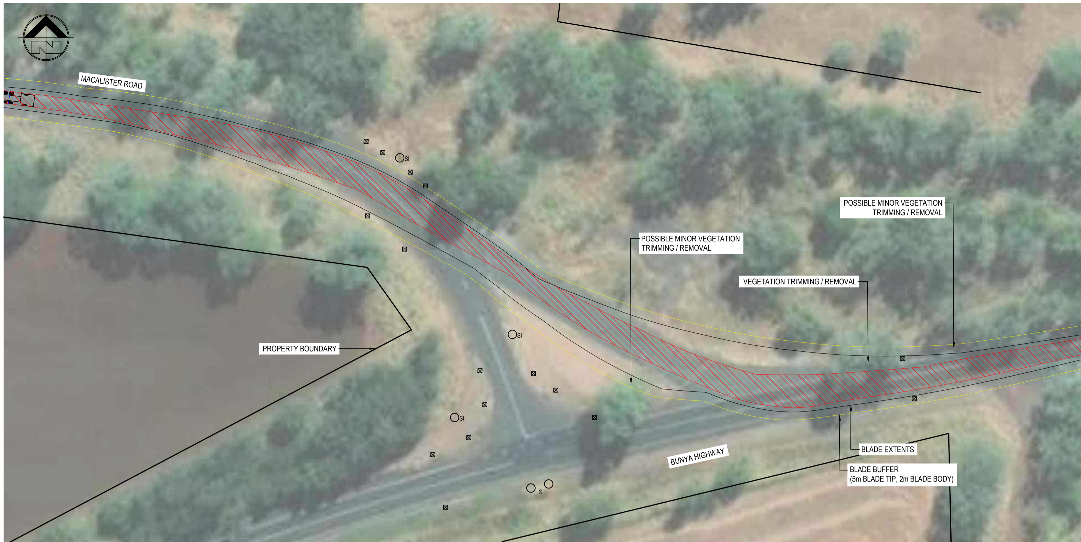
INTERSECTION 13 - MACALISTER ROAD / BUNYA HIGHWAY INTERSECTION PLAN - 90m BLADE TRUCK AND TRAILER SCALE 1:500
