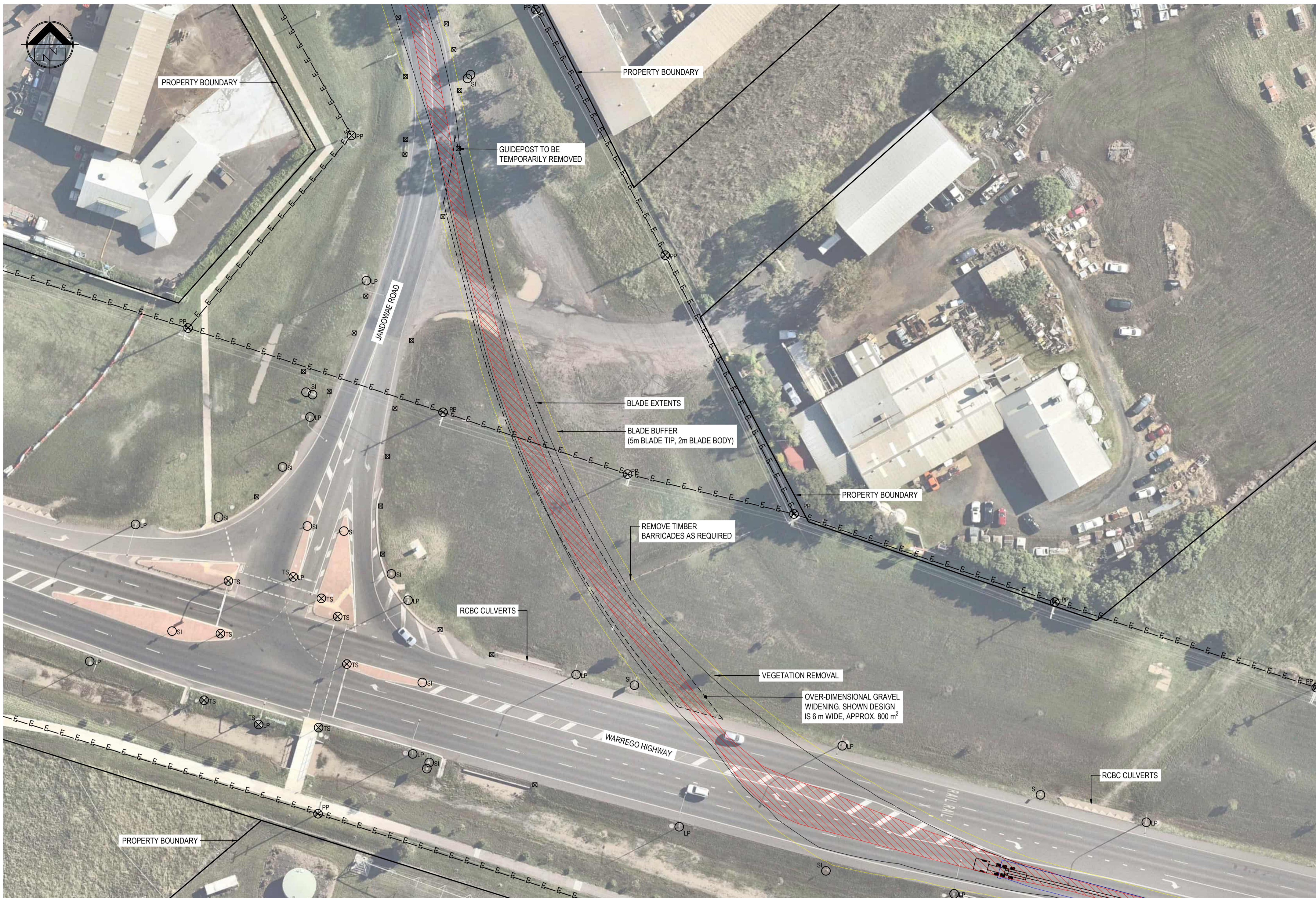
INTERSECTION 9 - WARREGO HIGHWAY / JANDOWAE ROAD INTERSECTION PLAN - 90m BLADE TRUCK AND TRAILER - OPTION A
